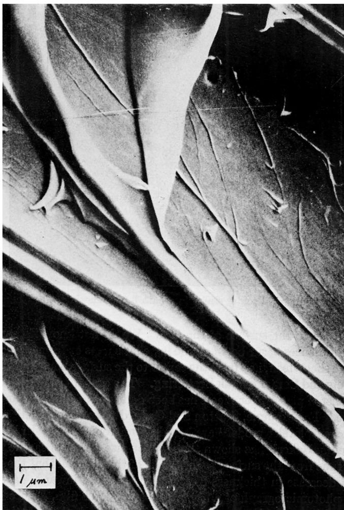
Fig. 10. Scanning electron micrograph of a fractured, biaxially oriented (path 3) film.
